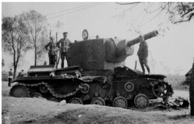
German military inspect the Soviet KV-2 tank with a broken chassis. Even without enemy shells, the overloaded KV-1 and KV-2 chassis often fail. Memories of German corporal Helmut Claussmann: «... Once in our division a soldier was shot, who wrote a defeat letter home in which he scolded Hitler. And after the war, I learned that during the war years, for such letters, several thousand soldiers and officers were shot! One of our officers was demoted to the rank and file for „defeatist talk“. Especially feared members of the NSDAP. They were considered informers, because they were very fanatically minded and could always submit a report to you on command. There were not very many of them, but they were almost always not trusted. Attitude to the local population, to the Russians, to the Belarusians was restrained and suspicious, but without hatred. We were told
